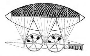
The parachute propellers are mounted on horizontal reciprocating shafts, and open and close alternately, the said shafts being actuated by eccentrics on the paddle-wheel axles.
